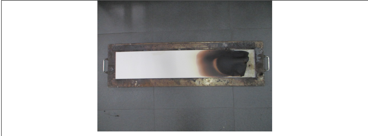
After test- Radiant heat source
